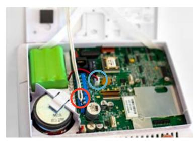
There are two wires you will need to remove: A. The power wire B. The battery wire
