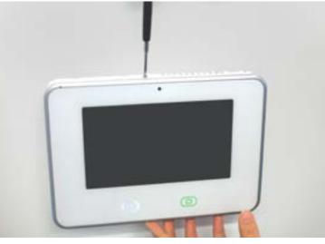
If your panel has a screw on the top, remove it with a crosshead screwdriver so that you can remove the panel cover. To remove the cover, push the two tabs on top and pull the cover out and down. Don't be alarmed if you hear beeping.
