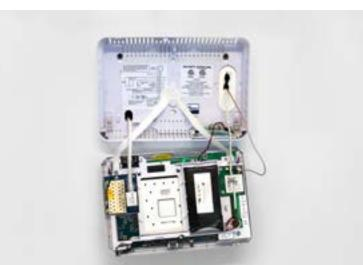
Hang the panel cover on the back plate using the white safety strip.
