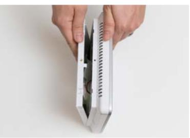
Reassemble your panel by snapping the front cover and backplate together and replacing the top screw.
