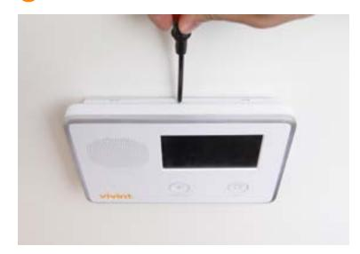
If your panel has a screw on the top, remove it with a crosshead screwdriver so that you can remove the panel cover. To remove the cover, push the two tabs on top and pull the cover out and down. Don't be alarmed if you hear beeping. 4
