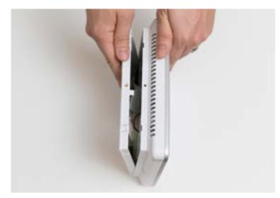
Reassemble your panel by snapping the front cover and backplate together and replacing the top screw.
