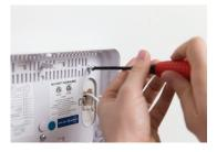
Remove all the screws from the backplate and remove the backplate from your wall. Please note there will be a small hole in the wall.
